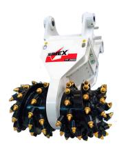
Simex rotary cutters are ideal for trench cutting on hard and compact materials, concrete or rock wall profiling, quarry works, demolition work, and dredging. The dual-head drum cutter features an internal hydraulic piston motor that provides direct power to the cutting drums for maximum efficiency and minimum non-operational space between cutters.
